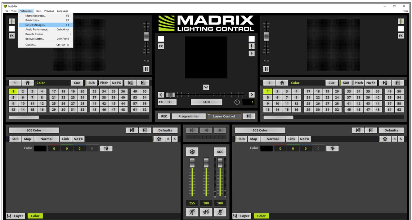
2 After we opened the **Device Manager** the **DMX Devices** tab is selected by default. If we have connected the MADRIX interfaces via USB before we start MADRIX, the interfaces will be found automatically.
