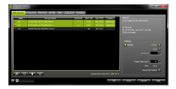
[In the screenshot above, one STELLA is connected. If more devices are connected, please use the different IP addresses of different devices to identify them in the Device Manager. You can also click on *Device Name* as well as *Universe* or other columns to sort the list accordingly.]
