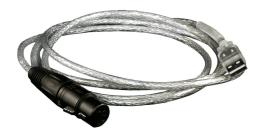
MADRIX USBone is a USB 2.0 DMX512 interface. It can be used for input [DMX-IN] or output [DMX-OUT]. The MADRIX USBone allows you to control 512 DMX channels using MADRIX. But an additional MADRIX KEY [i.e. a software license] is necessary.
