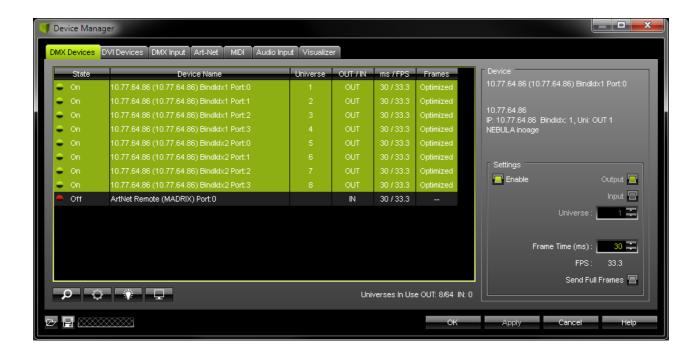
• [In the screenshot above, one NEBULA is connected. If more devices are connected, please use the different IP addresses of different devices to identify them in the Device Manager. You can also click on **Device Name** as well as **Universe** or other columns to sort the list accordingly.]
