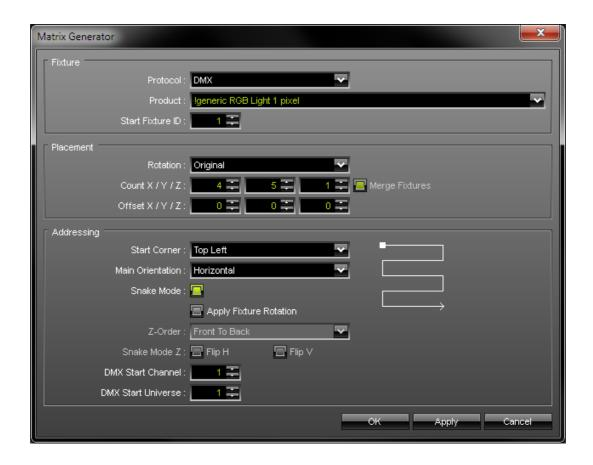
• In theory, the LEDs are arranged as follows: 3 pixels per LED [due to RGB], 4 fixtures per row, and a total of 5 rows. Please see the picture below:
